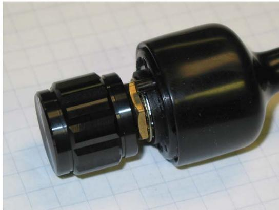
This switch has the capability of having 1 to 6 positions, depending on the index tab.
