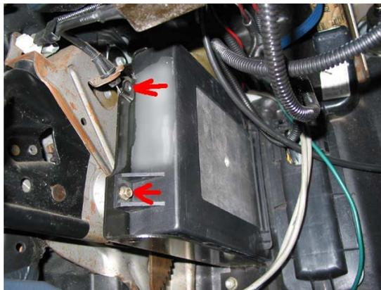
There are two 7mm bolts holding the black plastic computer sleeve to the metal computer-mounting bracket at the rear of the computer. Remove these first. Pull the plastic PCM cover towards the right about 2 inches out. Then pull towards you. The PCM should come out easily. If not, open the plastic box up a bit more. Note how the computer is oriented in the black plastic sleeve for reinstallation purposes later.
