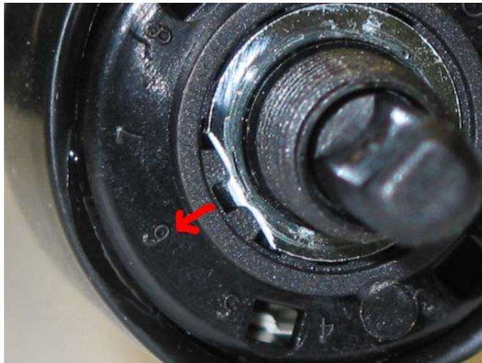
The above picture shows the tab of the index ring in the #6 index hole, allowing for 6 positions.
