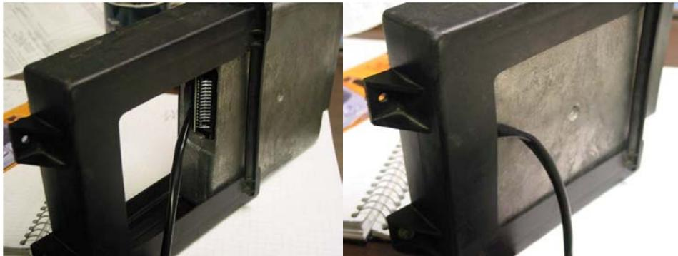
Make sure that you run the switch cable from the chip under the chip when you put the pcm back in the black plastic cover. You can cut a slot in the plastic cover to allow the switch wire to gain additional length if necessary.
