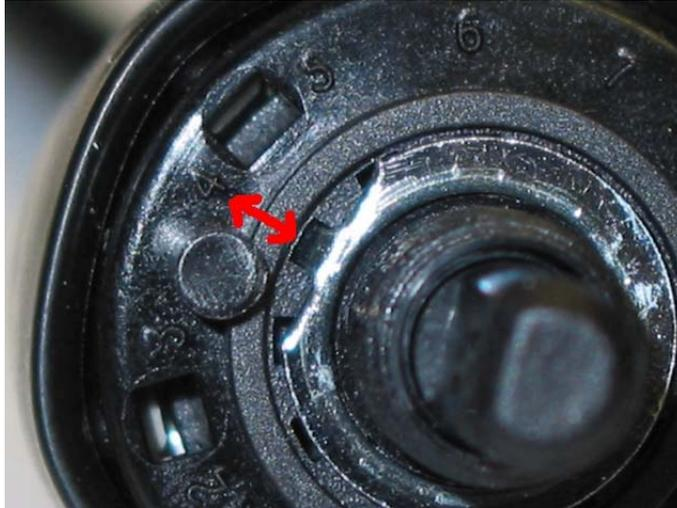
The above picture shows the tab of the index ring in the #4 index hole, allowing for 4 positions.
