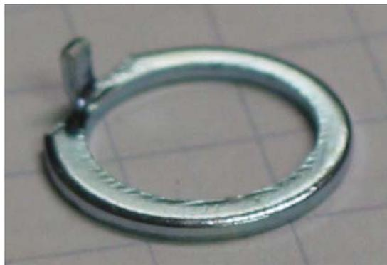
The index tab is placed in reference holes in the switch to coincide with the given amount of programs programmed in to the chip.
