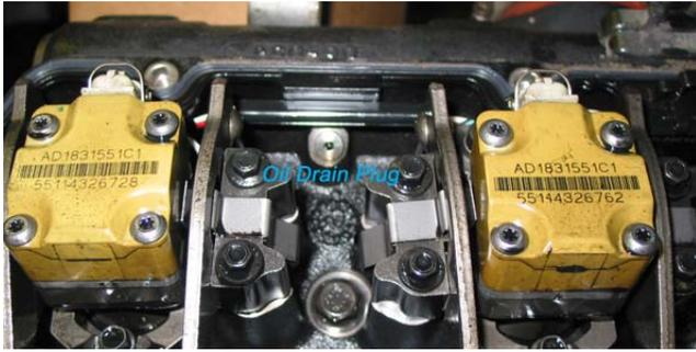
9. With a 8mm socket remove the bolt located on the fender side of the injector that holds the injector-retaining bracket down.
