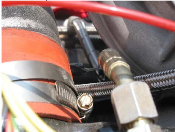
5. Once the hose is in place, double wrench the adapter and hose and tighten. **Note** – Make sure that the hose does not come in contact with the turbo housing.
