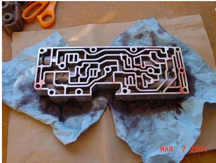
Towards the front of the transmission and running the entire width of the transmission is the accumulator valve body. It is held by two nuts (10 mm) and eleven bolts (8 mm). Unscrew the bolts and nuts from the valve body and lower it carefully as some remaining transmission fluid will spill out.
