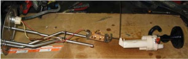
10. Loosen the hose clamp from around the top of the black rubber pickup foot and remove it from the white mixing valve.
