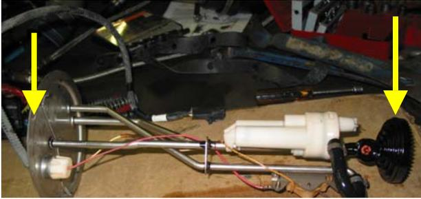
9. Remove the white mixing valve from the sender by first removing the rubber hose by cutting off the 2 metal band clamps then gently twisting off the 3/8" steel line.
