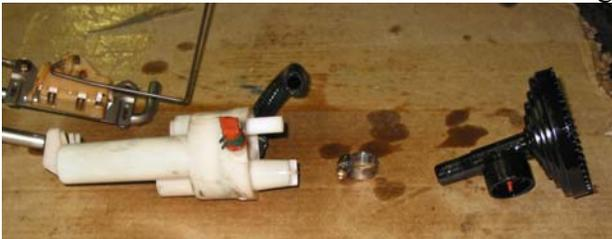
11. Remove the metal filter screen from the bottom of the black pickup foot. Using a drill and 3/8" drill bit, drill out the center of the black foot to remove obstructions. (What you see in the picture is the black foot drilled out and the pickup screen back in place)
