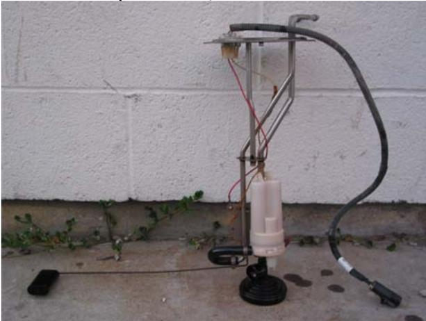
8. Measure the distance from the bottom of the pickup to the bottom of the flange. The distance should be around 15 1/4" for long beds and 13 3/4" for short beds.
