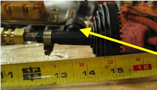
**CAUTION** – If you cut the tubing too short, you will suck air through the check valve in the side of the pickup foot. The tubing **MUST** be pushed past this point in the black pickup foot.
